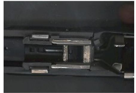
Cracked Receiver and Locking Block
