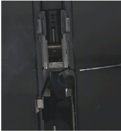
Cracked Receiver and Locking Block
